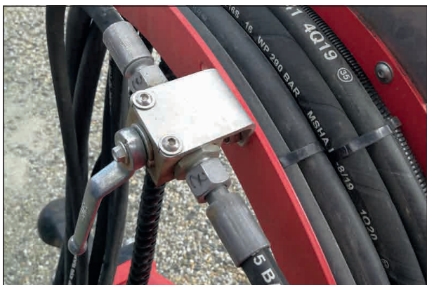
trailing steering axle lock valve closed (parking position)
