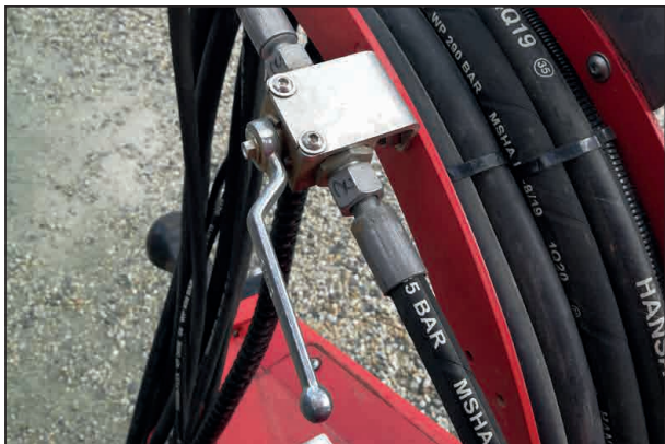
trailing steering axle lock valve open (field travel)
