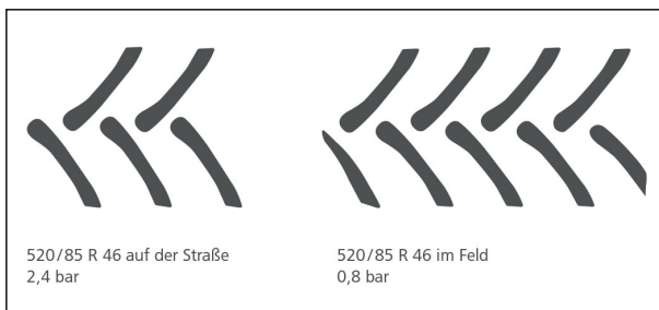
Tyre ground contact area depends on the tyre pressure
