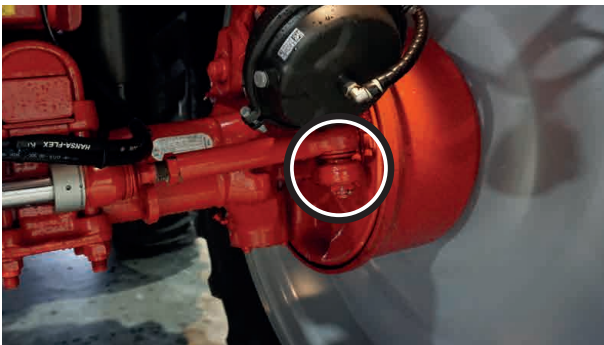
Tapered bolts on steering cylinder
