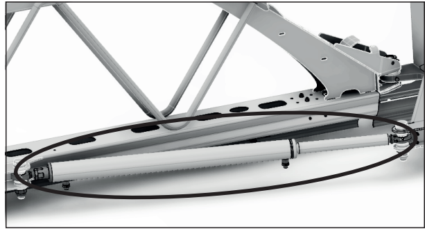
Folding cylinder with MotionControl (figure similar)
